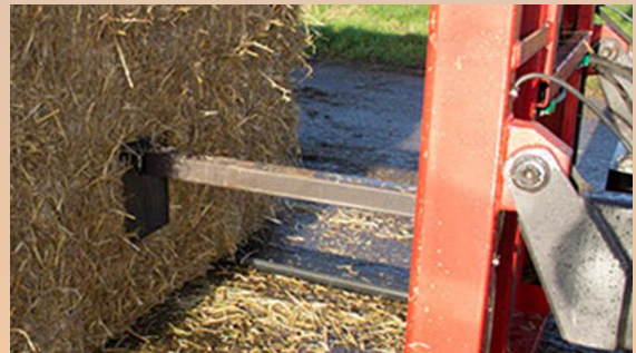
A special push-off mechanism makes it easy to pull out the forks from underneath the stack no matter if the surface is of soil, cement or asphalt.
