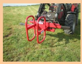
Bale grab for 9 bales - the ideal solution where efficient handling of easy-to-handle 15 - 50 kilo mini bales is required.
