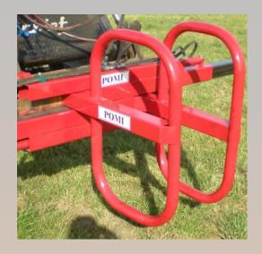
The bale grab is switch-controlled from the tractor - continuously variable setting option for grab from 400 to 2000 mm.
